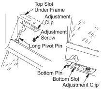
Figure 21 - Installing Glass Doors
